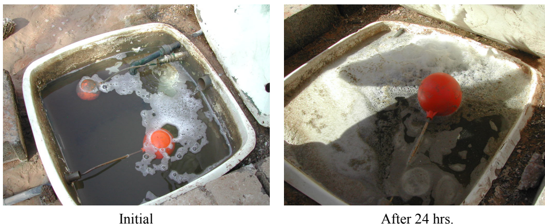
Figure 2. The effect of acidified water in removing scales and salt deposits from the cooling pad (dissolved salts in the reservoir of the cooling system).
