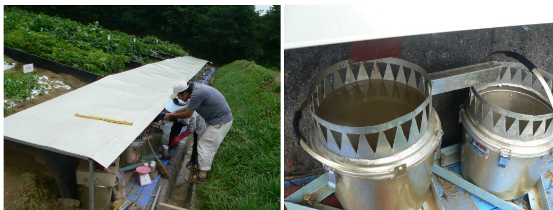
Figure 1. Simple soil loss and runoff collector installed in the plots.
